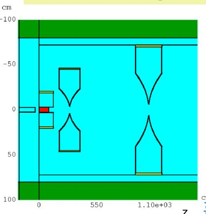
Target integrated into Horn 1 Assuming target radius of 0.9 cm
