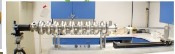
J-Lab : Lab cavity inspection tool based on long-distance microscope, Kyoto Camera
