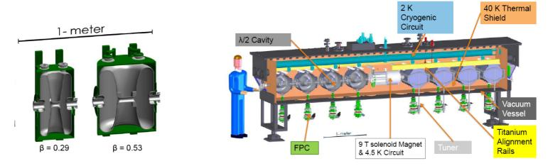
FRIB HWRs and  $\beta$ =0.53HWR cryomodule (courtesy of MSU-NSCL)
