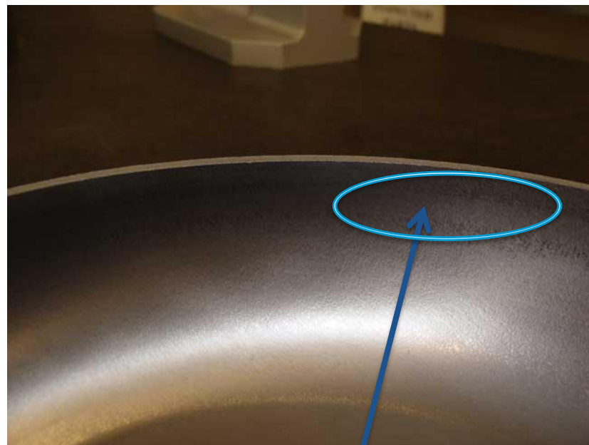
Equator thickening resulting from forming Increase in thickness of 10%
