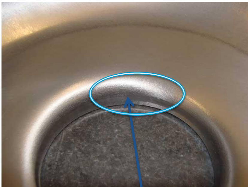
Iris compression/ thinning resulting from forming Decrease in thickness at Iris ~15%;
