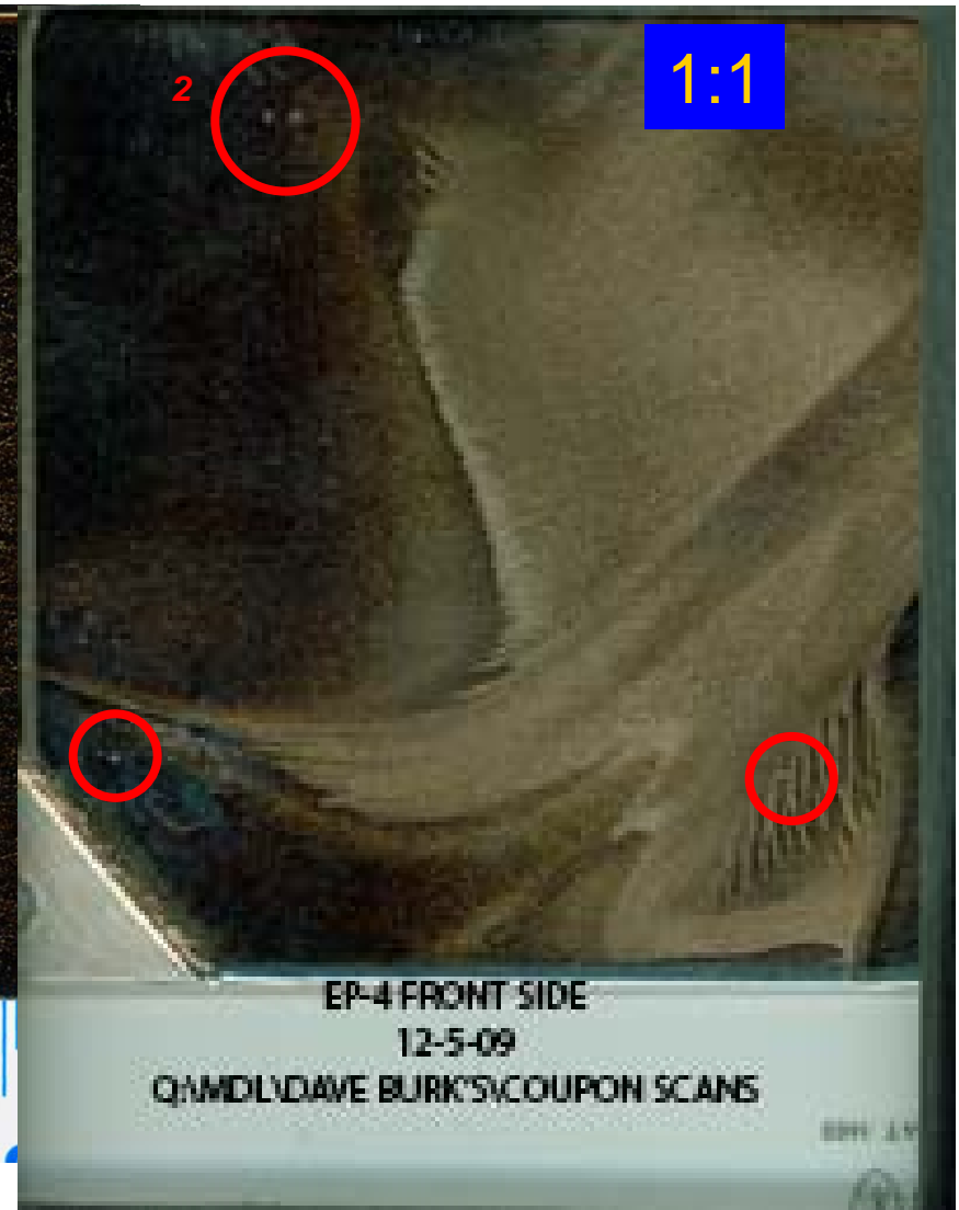
EP-4 31 °C 120 min, 160 \mu\text{m} removed 456 GU 110 nm Ra 4 pits / 50 \text{cm}^2 1:1 anode:cath
