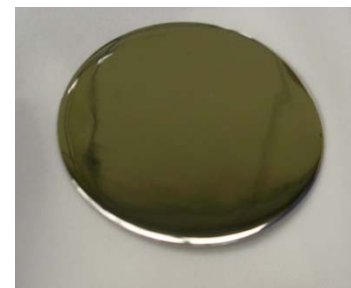
Single-crystal Nb substrate after 150 \mu\text{m} BCP
