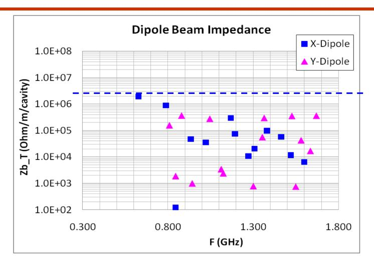
Dashed line is the beam instability requirement for dipole modes
