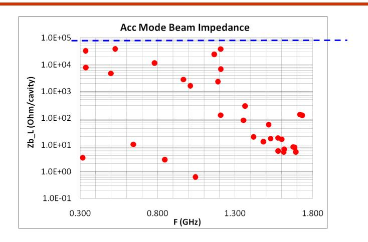
Dashed line is the beam instability requirement for accelerating modes
