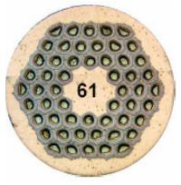
Compare with Ti-doped RRP-54/61 (Nb-2.0a%Ti)<sub>3</sub>Sn (Ti introduced by distributed Nb-47Ti rods in the Nb-Cu matrix)
