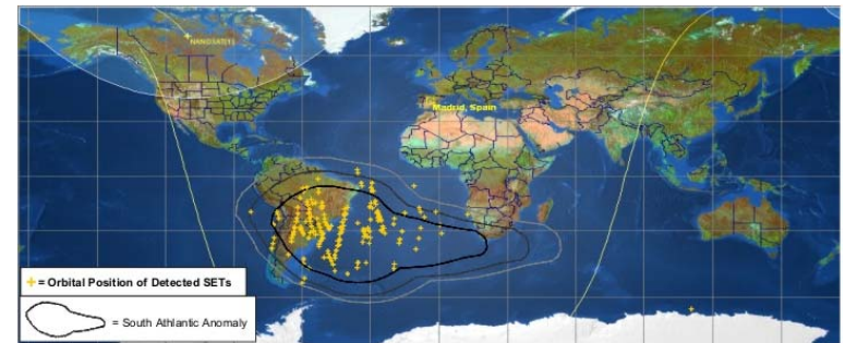
SET events experienced in Nanosat-1B. Courtesy of INTA Optoelectronics Lab
