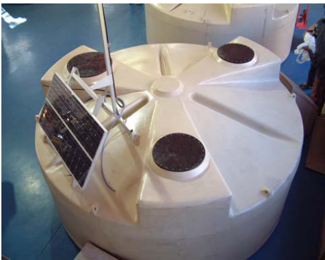
Auger South Tank 3 PMTs
