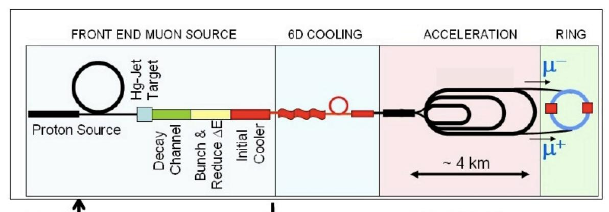
Proton source: Upgraded PROJECT X (4 MW, 2±1 ns long bunches)
