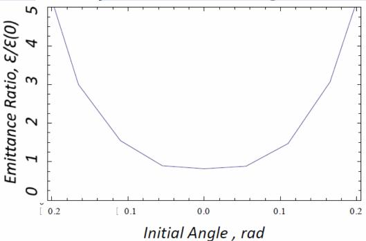
Emittance out for pencil beam (zero initial emittance), as a function of initial angle.
