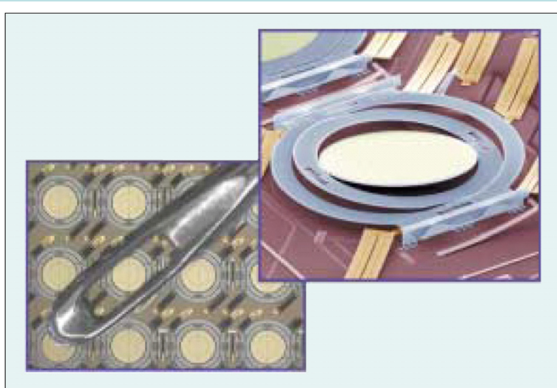
Figure 4. Two images of MEMS-based OXC mirrors used in the Lucent LambdaRouter. The image in the upper right is a single mirror, and an array of mirrors is shown in the lower left. An eye of a needle is shown for comparison on the array.
