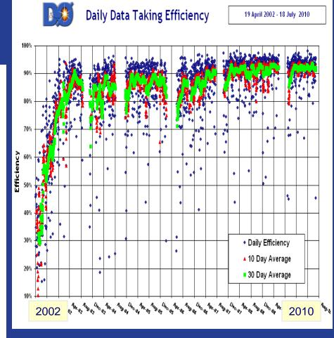
DØ is collecting data with over 90% data taking efficiency
