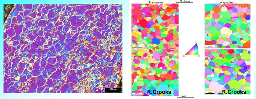
Microstructure and texture of Nb tubes produced by combination of spinning and flow forming
