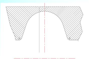
Nonsymmetrical mould for hydroforming
