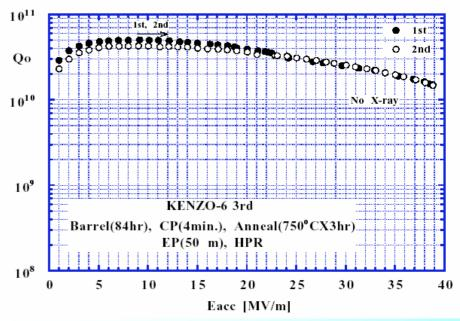
Some best seamless single cell cavities. Preparation and RF tests: K.Saito, P.Kneisel
