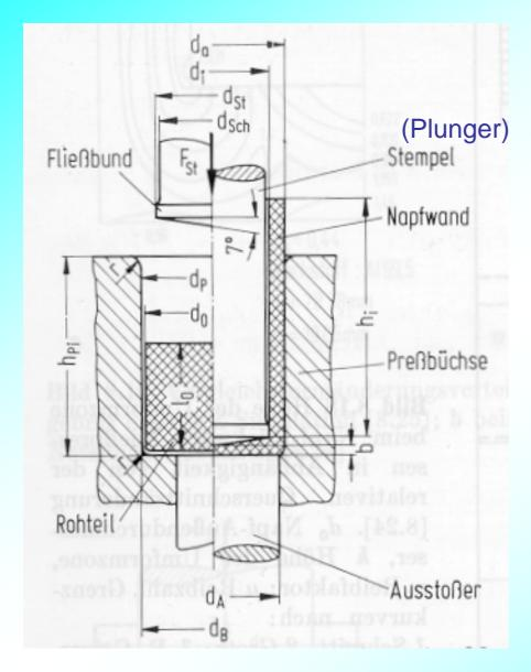
Principle of seamless tube fabrication by back extrusion
