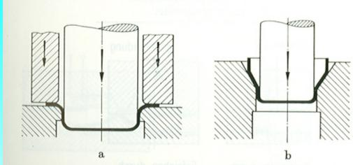
Principle of deep drawing; a-first step, b-second and further steps
