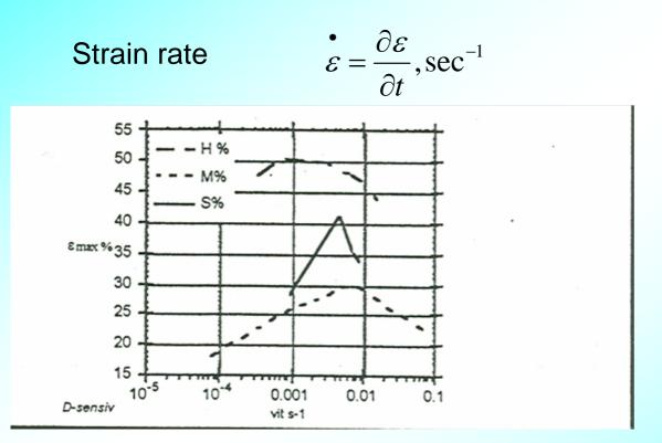
Dependence of maximum elongation of niobium versus strain rate (H, M, S different literature data).
