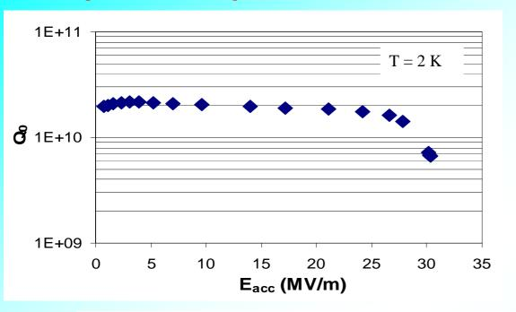
Surface treatment at DESY: 40 µm BCP, 800 °C heat treatment, tuning; 170 µm electropolishing (EP), ethanol rinsing, 800 °C heat treatment; 48 µm EP, HPR, assembly and evacuation
