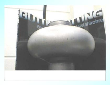
Single cell cavity fabricated at Fa. Butting (Germany) in collaboration with DESY from deep drawn tube produced at the company B.J. Enterprise (USA) (reached 39 MV/m
