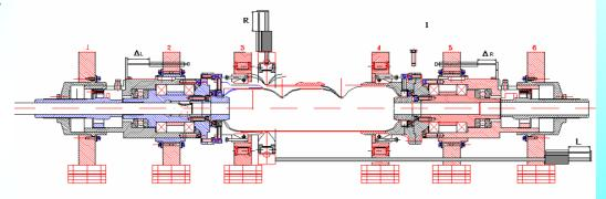
Principle of DESY necking equipment
