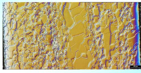
Microstructure of back extruded Nb tube produced from a pill taken from ingot
