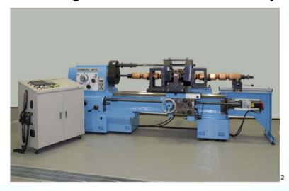
KEK necking machine (successful on Cu-tubes)
