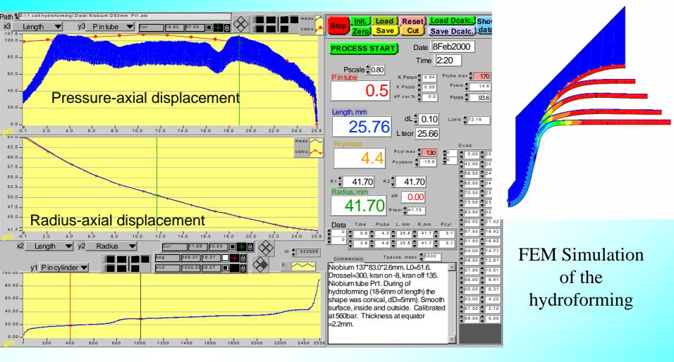
Front panel of the software for hydroforming - machine
