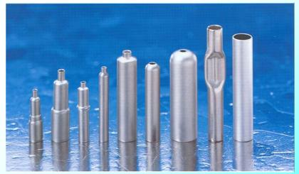
Different tubes with covers from Nb1% Zr produced by back extrusion at the company W.C. HERAEUS (Germany)
