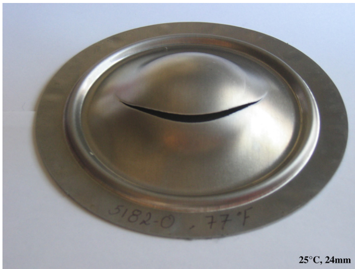
Fig. 15. Pure stretch experimental results using the 101.6 mm (4 in.) hemispherical punch at 25 °C (77 °F) for AA5182-O. Punch depth at failure is shown.
