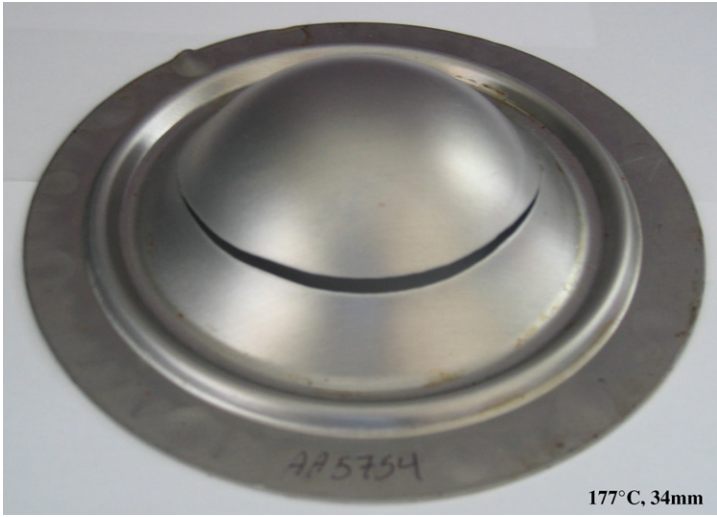
Fig. 20. Pure stretch experimental results using the 101.6 mm (4 in.) hemispherical punch at 177 °C (350 °F) for AA5754-O. Punch depth at failure is shown.
