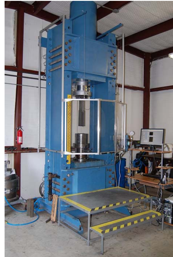
376 Ton, 40" stroke, instrumented hydraulic press
