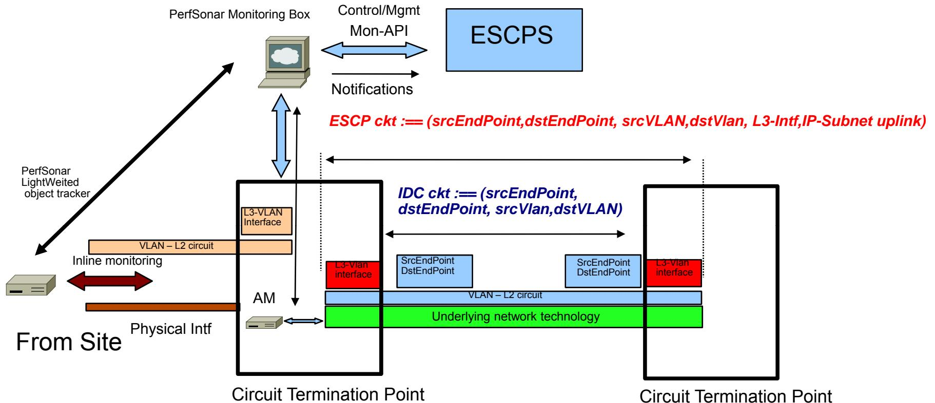
AM – Active measurements from the inside of Termination Point
