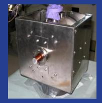
Development and fabrication of splittable quadrupole (ID=78 mm, G=54T/m) with indirect coil cooling for installation in SCRF cryomodule.
