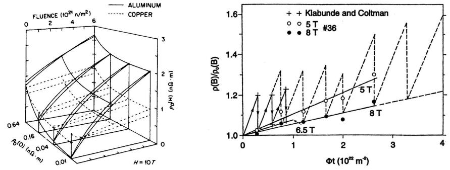
Annealing by cycling to room temperature gives essentially complete recovery of the low-temperature resistivity of Al, but only about 80% recovery for copper.
