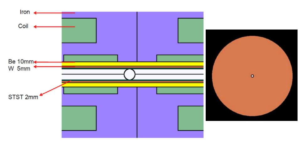
Liner + W collimator (2.6 cm aperture)
