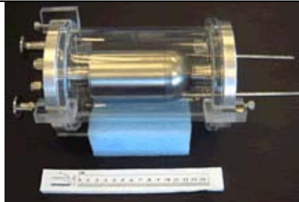
A cylindrical neutron generator configured to approximately 20 cm in length.
