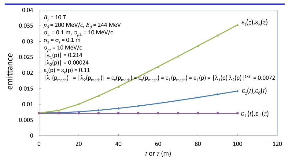
The transverse emittance is completely stabilized by an axial magnetic field. It makes no difference whether canonical momentum p or mechanical momentum  $p_{mech}$  is used in the calculation of  $\varepsilon_{\perp}$ , although  $\varepsilon_x = \varepsilon_y$  are large when using p (but do not grow with t or z).
