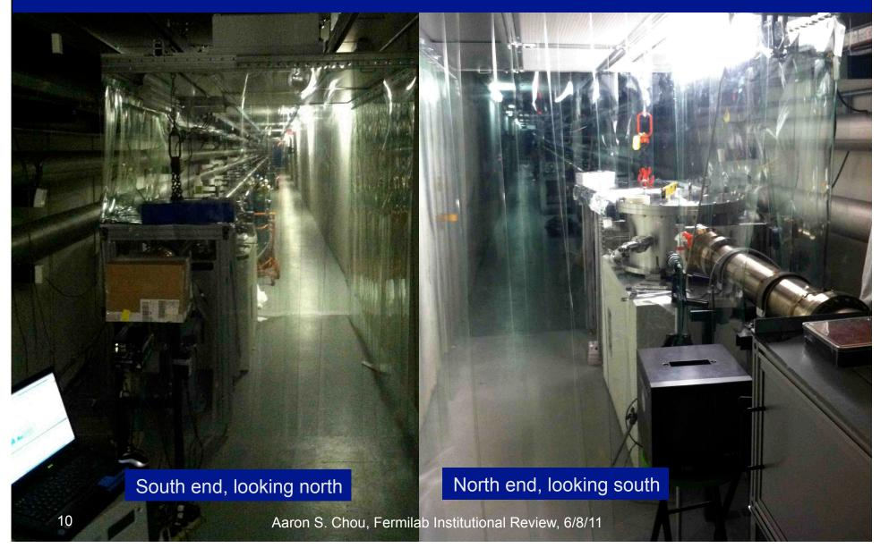
End station vacuum vessels hold custom optical cavity mirrors and eventually beamsplitters
