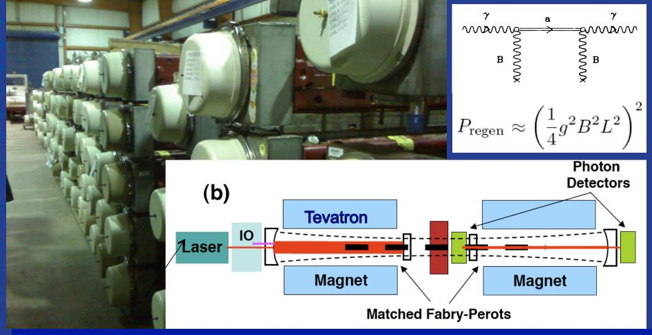
Increase photon flux from  $10^{19}$  to  $10^{24}$  γ/s, increase L from 6 to 40m, resonantly detect  $\rightarrow$  improve laser axion sensitivity by 4 orders of magnitude.
