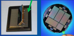
CCDs, wafer from LBNL, packaged at FNAL
