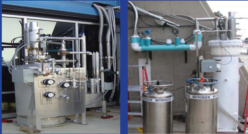
Cooling and Vacuum System, FNAL , Keep CCDs at 173K, 10^{-6} Torr
