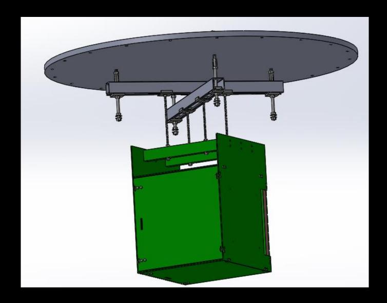
Mounts with 3/8" Threaded rod & Stainless Steel Unistrut
