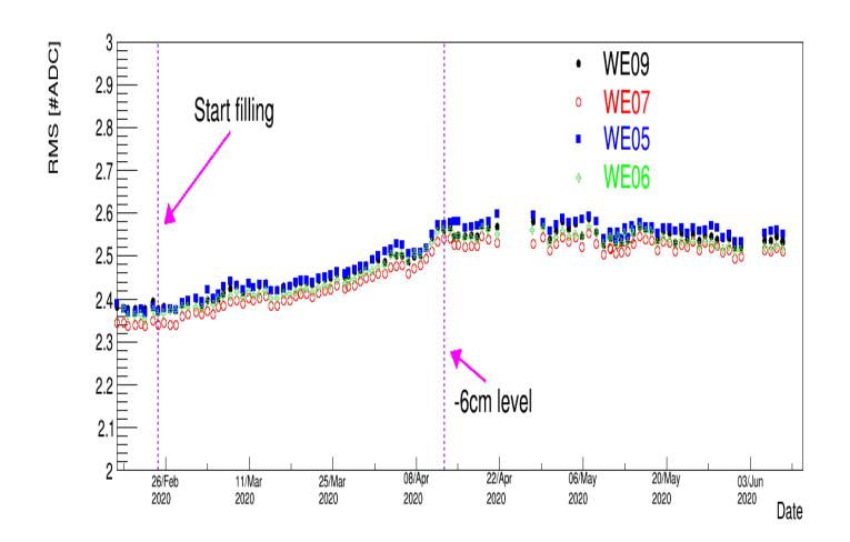
A gradual increase of the intrinsic noise in +/- 60° TPC Coll. and Ind.2 wires with the LAr level corresponding to ~35 pf increase of the wire capacitance is observed, in agreement with the expectations.
