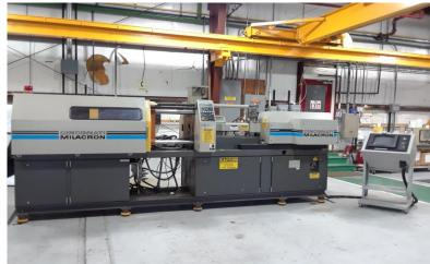
Injection molding machine at Lab 5 will be used to make the voxels.
