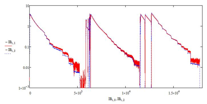
Beam current from DCCT & WCM for 3 measurement of March 6 (2 uncoupled & coupled)
