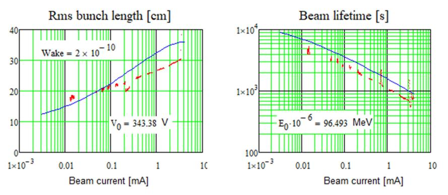
Measured L<sub>bunch</sub> at small currents is larger than the model predicts
