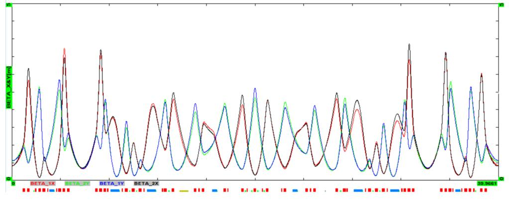
After careful decoupling, the coupling was introduced by SQA1L, GdL= 200 G, Tune split: 0.015
