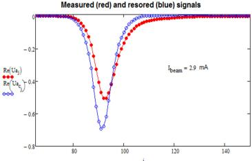
It starts getting non-gaussian tails and visible bunch self-compression with current increase
