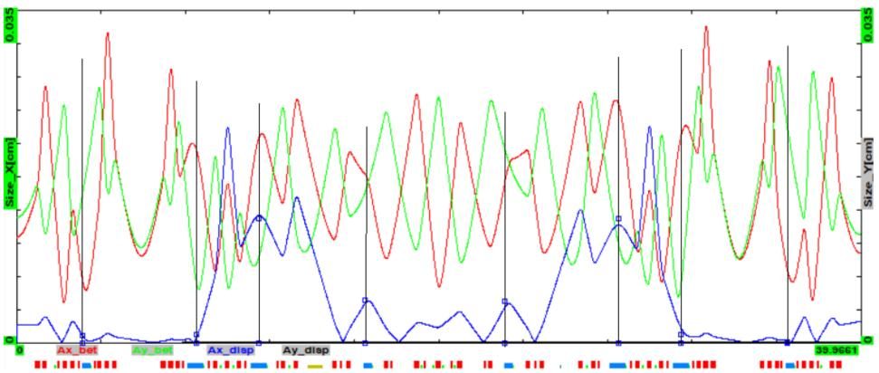
Rms bunch sizes for small beam current (SR driven, no IBS). Vertical lines mark sync-light locations
