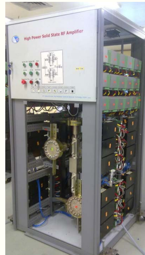
8 kW, 505.8 MHz Solid State Amplifier
