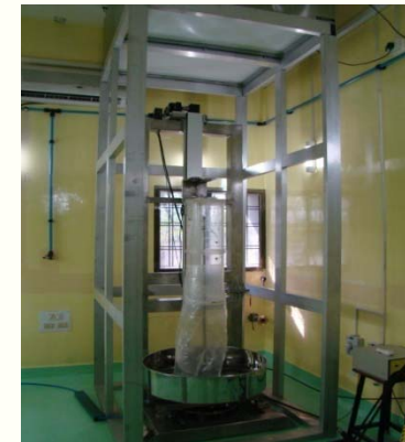
High pressure rinsing Set up
