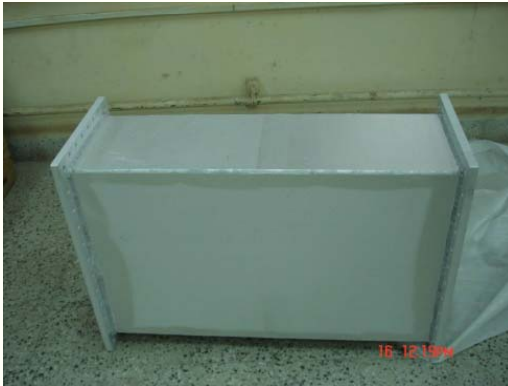
WR 2300 full height straight section
