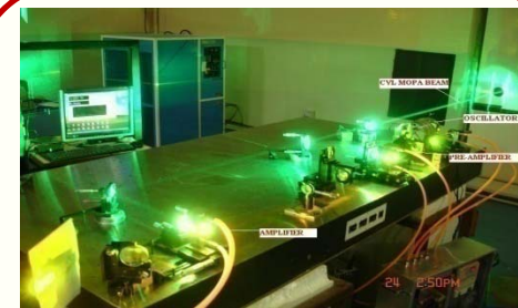
Single mode dye MOPA system and dye oscillator giving 1.1 watt average power at 200 MHz line width
