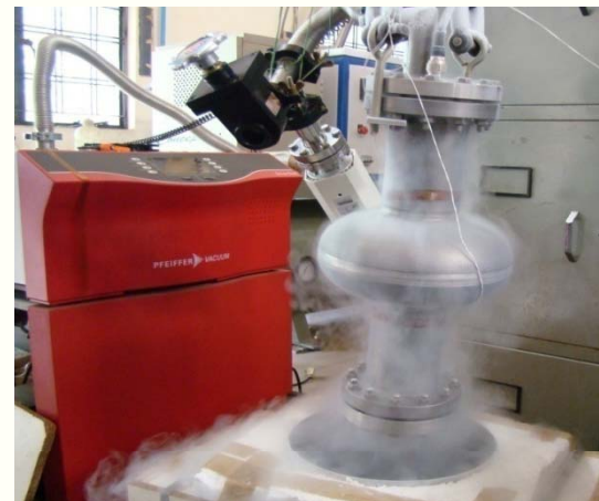
Leak testing of Single cell cavity at 77 K
