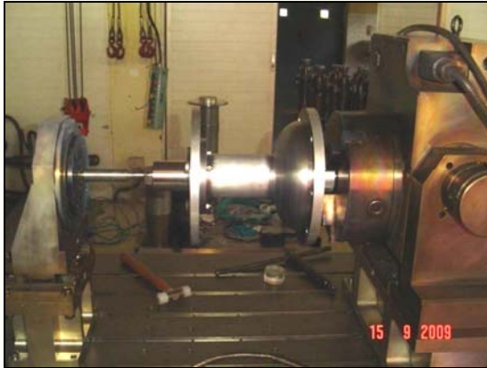
Outside iris welding
