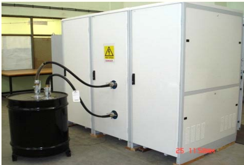
100 kV, 800 \mu sec pulse duration, 2Hz PRR solid state bouncer modulator.
