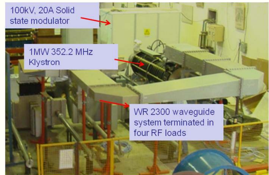
352.2 MHz, 1MW Pulsed Test Stand
