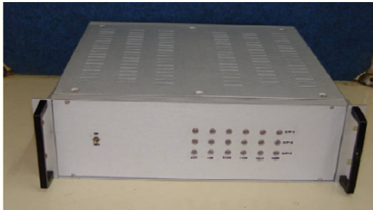
Multiple output DC power supply
