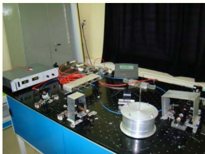
Fiber laser with 50W cw output power suitable for micromachining.
