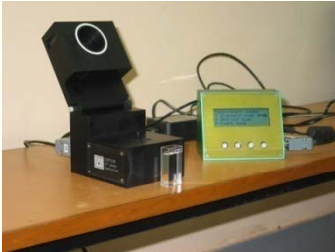
Laser Uranium analyser for glove box use
