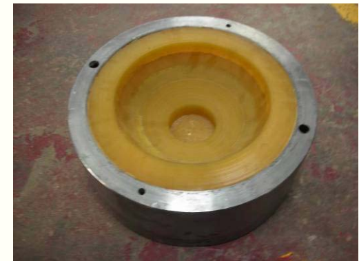
Improvement - rubber pad forming tooling completed
