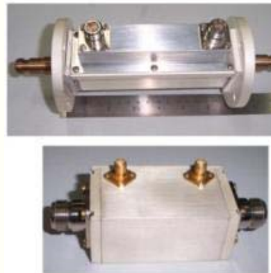
4kW & 1 kW Coaxial Directional Couplers
