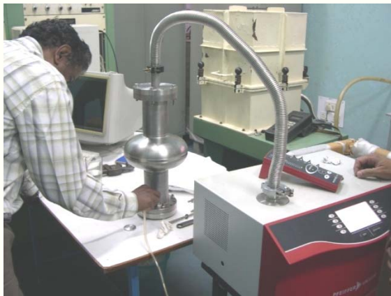
Leak testing of Single cell cavity at 300 K
