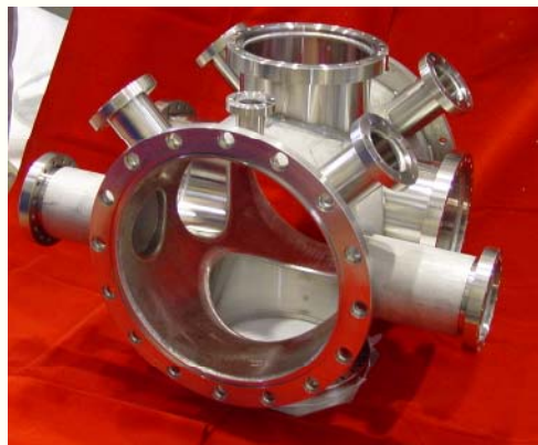
Beam extraction chamber
