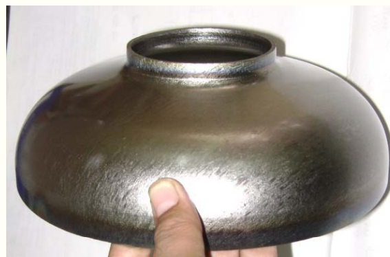
Formed Niobium Half cell
