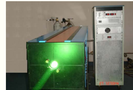
Copper Vapour Laser With solid state pulser, 40 W, 6kHz
