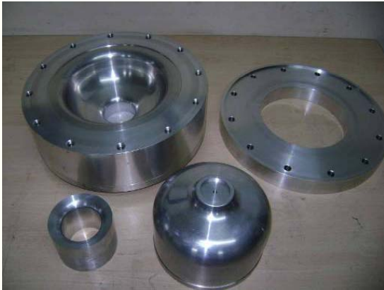
Half Cell Tooling (Aluminum alloy 7075-T6 from Fermilab)
