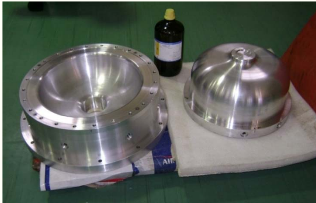
650 MHz cavity forming dies (Material Aluminum alloy 6061 – T6)
