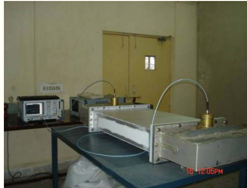
WR 2300 half height straight section
