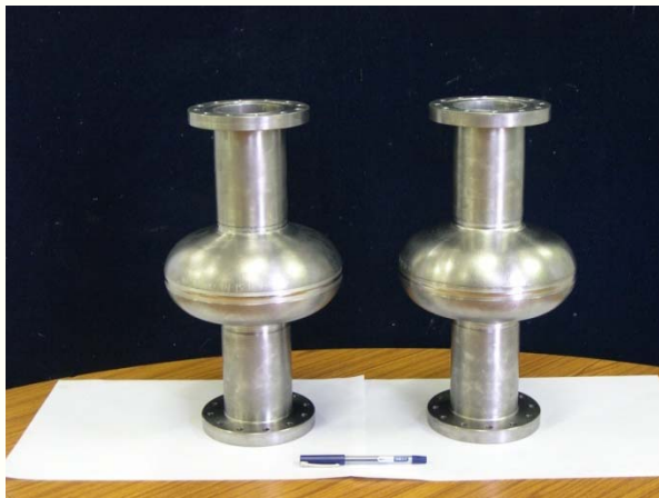
1.3 GHz Single cell Prototype cavities
