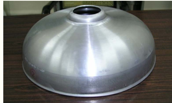
Prototype formed half cell in Aluminum (March 2011)
