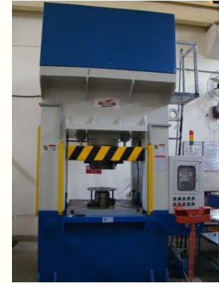
Cavity forming facility
