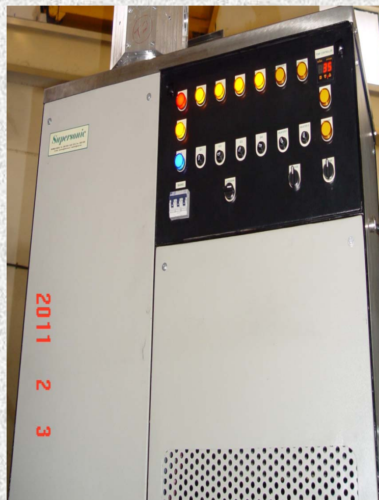
Ultrasonic cleaner for 9 cell cavities
