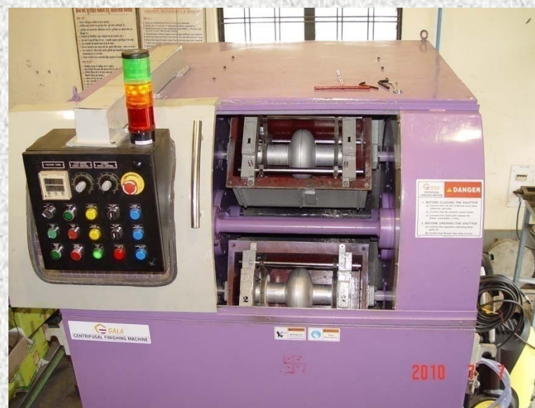
Cavities mounted in CBP machine
