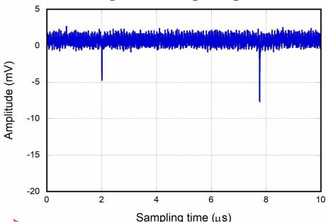
The amplitude distribution of these pulses will be used to monitor the gain stability of the tubes, while the frequency of the pulses will estimate the light background rate.
