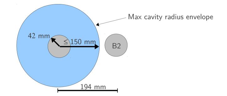
Both cavities fit in horizontal crossing (nominal configuration) Only works for CMS for the moment
