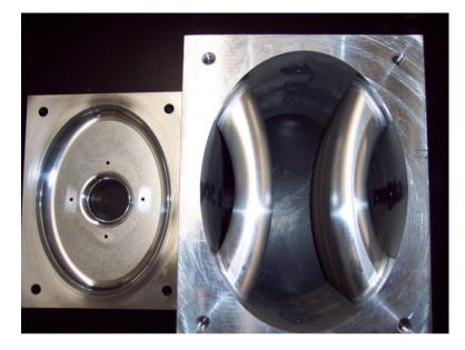
RF measurements on 800 MHz Al-model show precise frequency measurements for HOMs.
