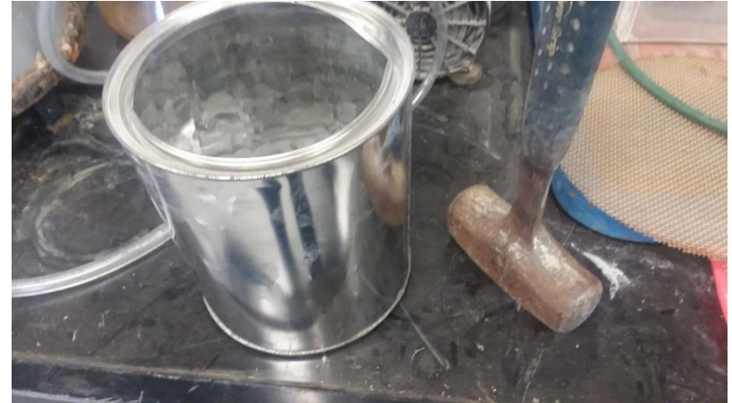
Bucket and mallet used to crush samples into small pieces.
