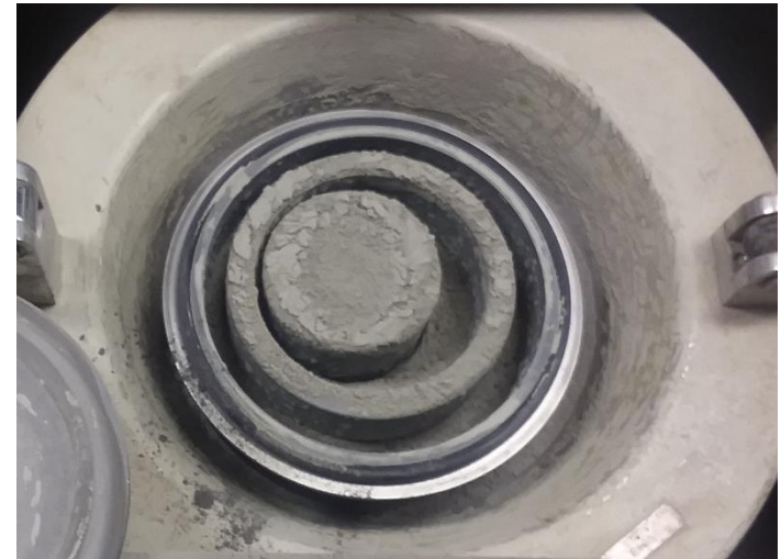
Milling machine with milled sample.
