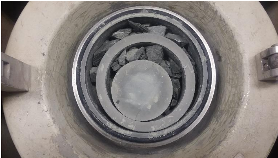
Milling machine with aggregate sample.
