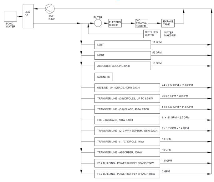
TOTAL FLOW REQUIRED - 315 GPM FLOW AVAILABLE - 400 GPM
