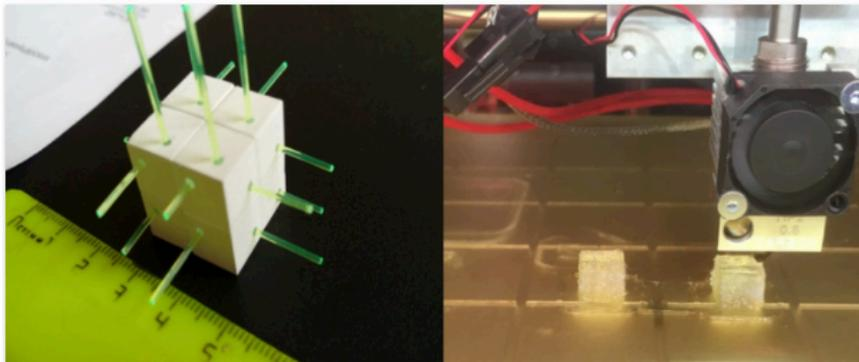
Example of a plastic Scintillator detector (left) and a stage of its 3D-printing process (right) (Image: CERN)
