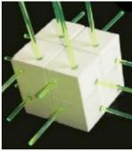
Injection molded scintillator for future high granularity experiments – Dune 3DST
