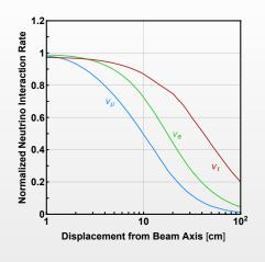
The neutrino interaction rate per unit area normalized to the prediction at the beam collision axis for a detector with radius 1 cm < R < 100 cm.
