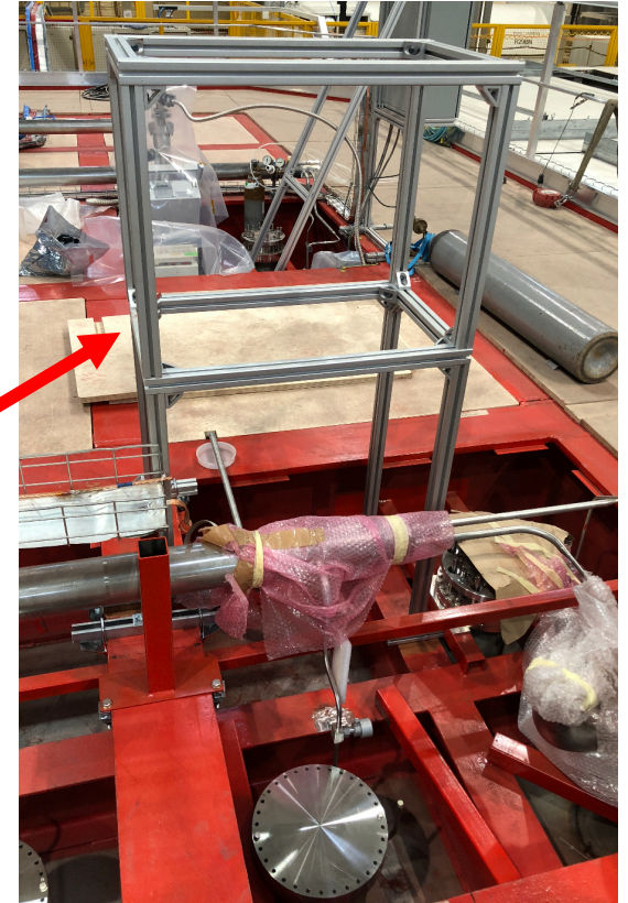
Rack for PrM Front-End electronics and Xenon Light source
