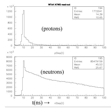
Velocity of MeV neutrons is  $\sim 0.05 \text{ c}$
