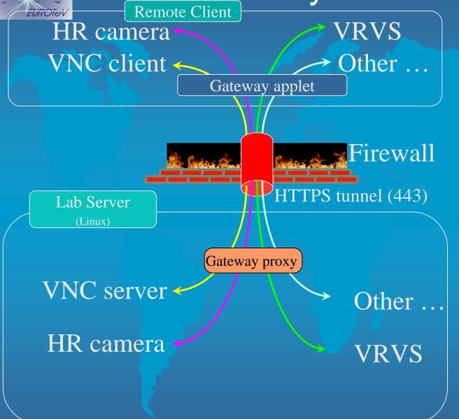
The Gateway proxy and applet allows us to tunnel all other ports through the ONE SSH-HTTPS port (443)
