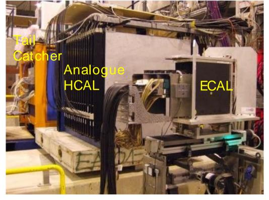
lated O(15000) calorimeter cells readout by Calice DAQ No Zero Suppression r/o speed 5 Mbyte/s continously IDTB Workshop Fermilab Jan. 2007 3
