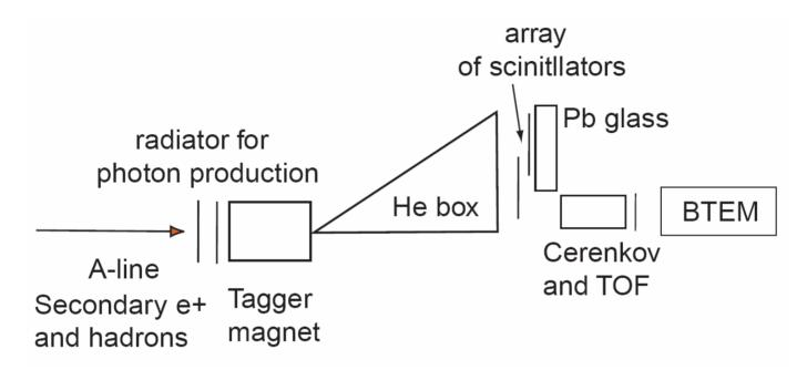
Beam setup for GLAST calibration a few years ago: Use a secondary positron beam Produce photons in a radiator inside of ESA Tag the positrons to measure the photon energy Calibrate your calorimeter with photons
