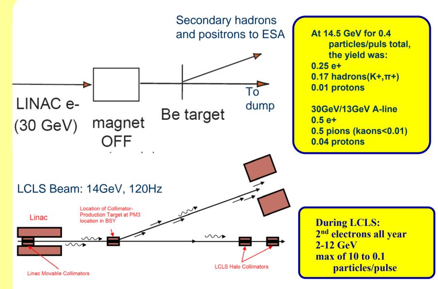
Test Beam Capabilities at SLAC
