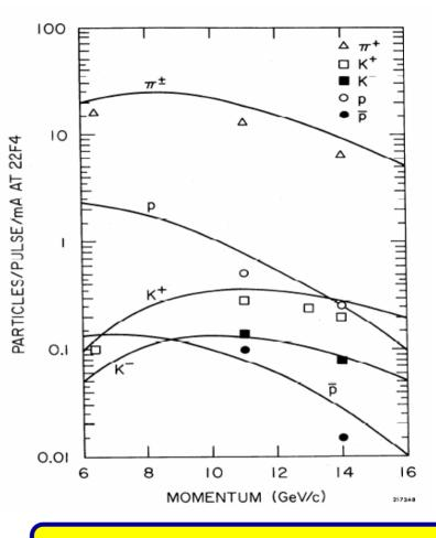
Primary beam energy is 19.5 GeV. Production target is 0.87 r.l. Be and production angle is 1.5deg. Momentum acceptance is +-2%  $\Delta p/p$ . Pulse length is 1.6 µs so that 1mA corresponds to  $1 \cdot 10^{10}$  electrons per pulse.
