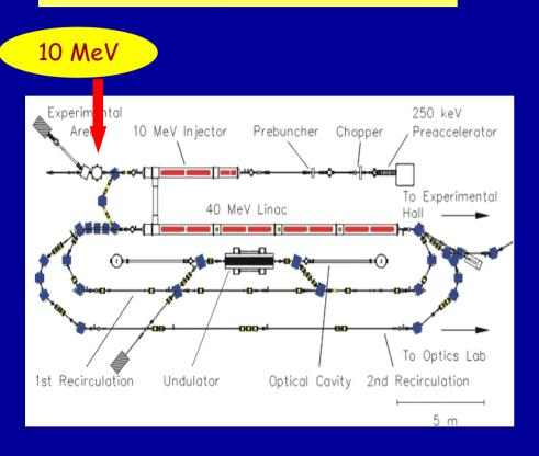
20-40 MeV Rooms FELA FEL3  $0.15-1.2 \, \mu m$ FEL1 1-6 um infrared Intector FEI with bunch 5-30μ Operation in fall 2007 compressor
