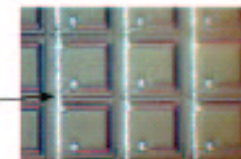
SiPM: pixel device operated in Geiger mode
