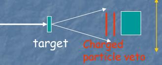
Moveable calorimeter to measure the rate and energy distribution of isolated clusters
