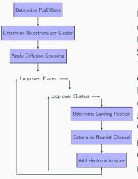
Landing positions are calculated and used to find the Nearest Channels. Electrons are collected and stored in SimChannels (per wire). The SpaceCharge module is used to deal with our non-uniform Electric field. But, we lose the 2D information (landing position), and so we can not apply correctly any gain variations. We also have difficulty with collection planes (correlation of number of electrons detected per cluster per plane).
