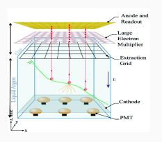
Dual-Phase has additional steps to Single-Phase LArTPCs. Electrons are extracted into the gas. In the LEM holes, Townsend avalanches occur. Electrons are collected on two split anodes.
