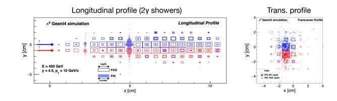
Studied in simulations 20 layers: W(3.5 mm  $\approx$  1X<sub>0</sub>) + silicon sensors Two types: Pads (LG) and Pixels (HG)
