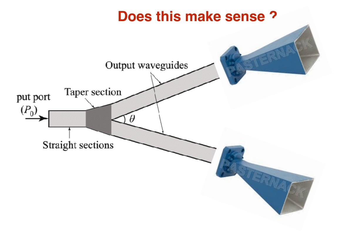
We can make it using horns and waveguides, so we could also make it using mirrors ...
