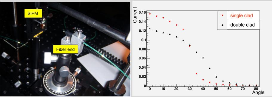
As expected, more light is trapped at higher angles for 1.2mm multi-clad fiber
